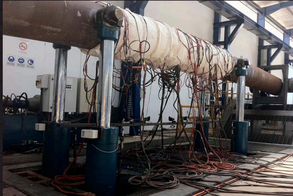
NPS 24 Lined Test Pipe Mounted on 4-Point Bend Test Rig
